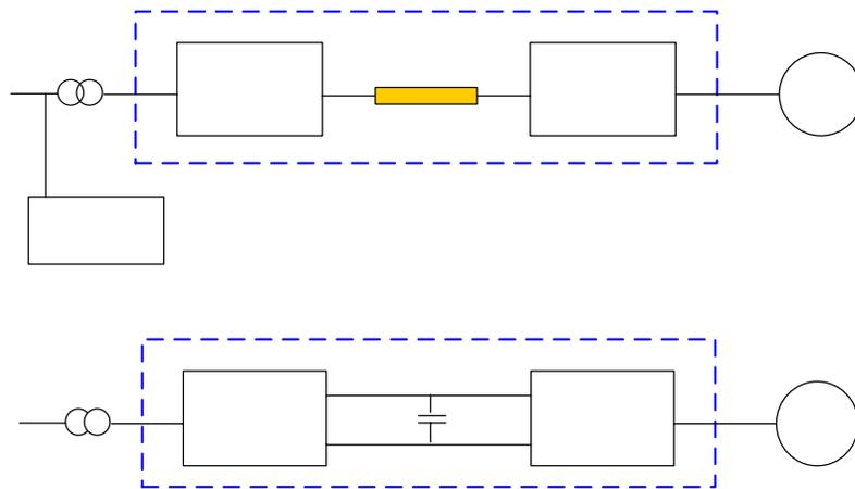
The LCI is a conventional drive system that uses a low switching (on/off) frequency device known as a thyristor. The GCT is a more advanced drive system that uses the latest high switching frequency device. Comparisons of these two technologies are presented in Table 1.
